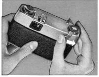
When loading the camera, the start of the film is wasted by exposure to light and so you must first make two blank exposures before starting to photograph.
