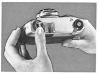
is complete and you can then open the camera. This is done by moving the catch on the base of the camera to "open" and then removing the camera back downwards. Put the cassette in its light-tight packing and mark it as exposed.
